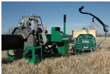
DynaMc 28 HP 2” IPS to 8” DIPS (63 mm – 225 mm)
