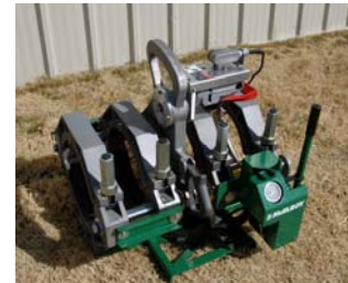
DynaMc 412 HP 4” IPS to 12” DIPS (110 mm – 340 mm)
