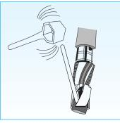
**Right**Coupon retained in cutter head after tapping.
