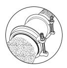
**STEP 6:** Positioning the Coupling. Once the gasket is properly sized, position the coupling over the pipe ends and cover the match-marks on the pipes. For uncoated ductile iron, grey cast iron and asbestos cement pipe surfaces, appropriate gasket lubricant is required on both gasket's inside surface and pipe's outer surface. Do not lubricate PVC, Steel or any PE pipe surfaces.
