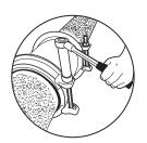
**STEP 7**:Tightening the end rings. Tighten the coupling bolts to the right torque shown on the product's label.
