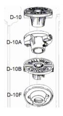
D-10 Regular ribbed cover and brass pentagon plug. D-10A Ribbed repair cover c/w set screw and brass pentagon plug. D-10B Ball valve marking ribbed cover and brass pentagon D-10C Cover and brass pentagon plug with seal. D-10D 11/4" ribbed cover and brass pentagon plug. D-10DR 11/4" ribbed repair cover with set screw and brass pentagon plug. D-10F Flat cover with 1" brass
