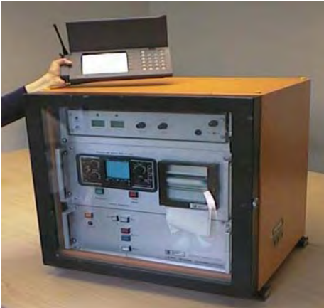
Figure 1, Leak Noise Correlator circa 1979.
