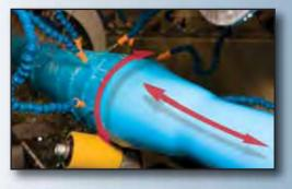
Stretching regular PVC pipe biaxially in both the hoop and axial directions—lengthways and sideways—over a mandrel after the pipe is extruded dramatically improves the performance of PVC material.
