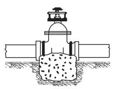
Install anchor rods around the valve body or through the mounting lugs and embed the rods in a concrete pour beneath the valve. Valves installed in chambers must also be anchored in this fashion. The critical time for restraint of valves is during opening or closing.
