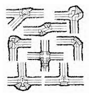
Typical thrust block locations. Trim the trench bearing area using hand tools to be sure of undisturbed soil.
