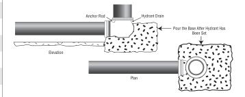
This type of hydrant foundation acts as a thrust-block, as an anchorage against frost heave and eliminates washouts from waste-water drain.
