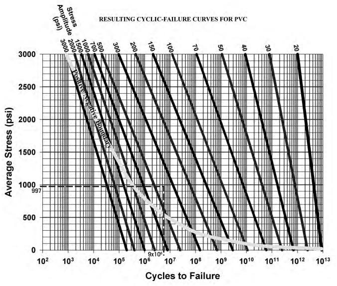
Determine the predicted number of cycles to failure using Moser's plot:
