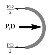
Referring to the Figure, we can see that the force in the pipe wall is:
