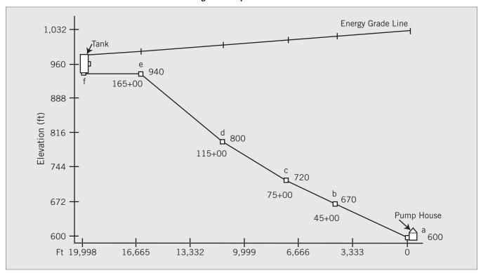
The objective of the design process will be to select proper DRs of PVC for appropriate sections of pipeline while never exceeding the PR nor the WPR of the pipe at any point. An effort will be made to select DRs that meet the design criteria while providing optimum economic value for the utility or owner.
