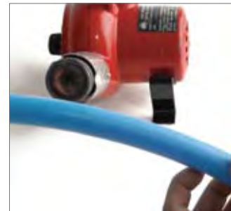
Repair kinks without cutting
